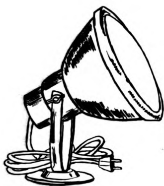
Enclosed floodlight, re- sistant to moisture, heat or cold. Lenses may be clear or colored.
