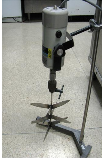
Figure 3.1. Modified servodyne mixer used to wash wheat bran. For interpretation of the references to color in this and all other figures, the reader is referred to the electronic version of this dissertation.
