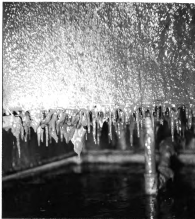
Figure 18. The Under Side of the Filter at the Hydraulic Load of 24.0 mgad.
