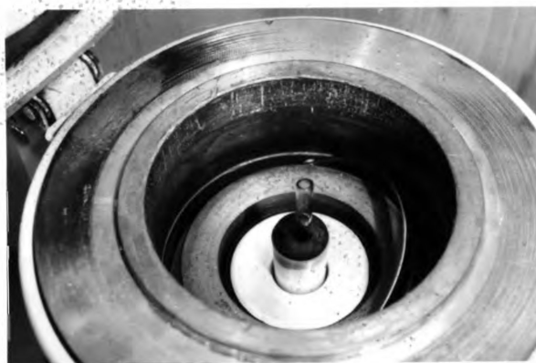
Figure 4. Detail of Scintillation Detector with Upflow Column in Crystal well.
