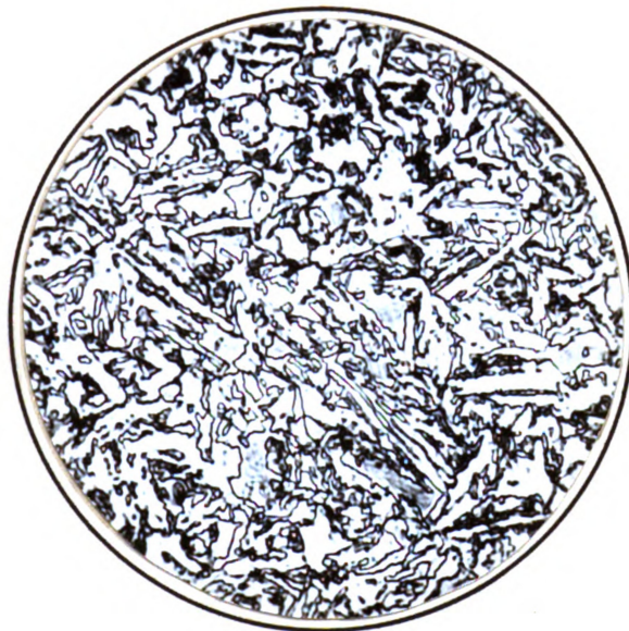
Figure 21 As received 2340 Steel Picral etch. 600x
