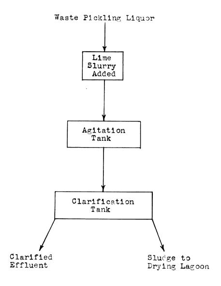
Flow-line Diagram Of Lime-Limestone
