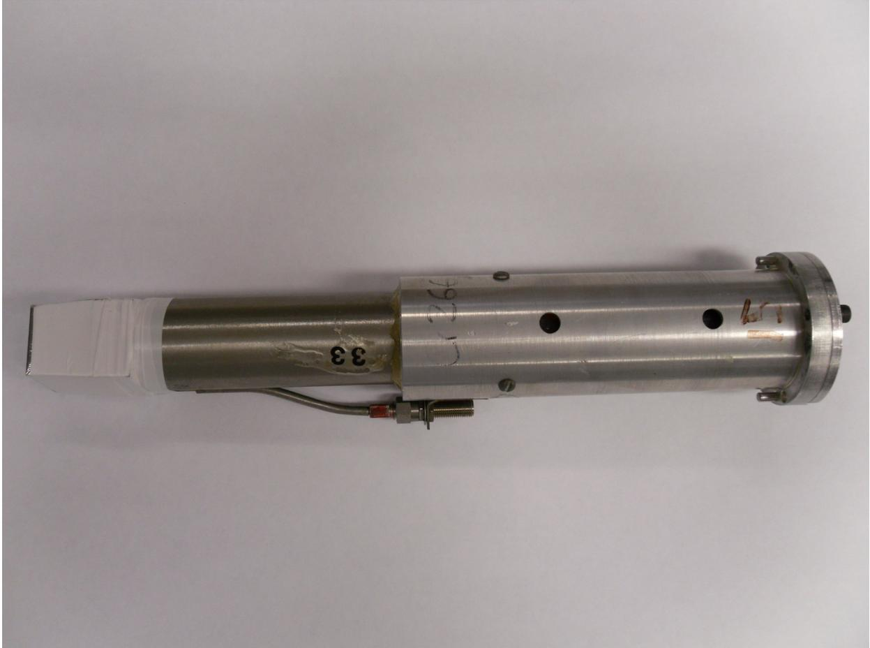
Figure 2.8: A picture of an individual Miniball element.
