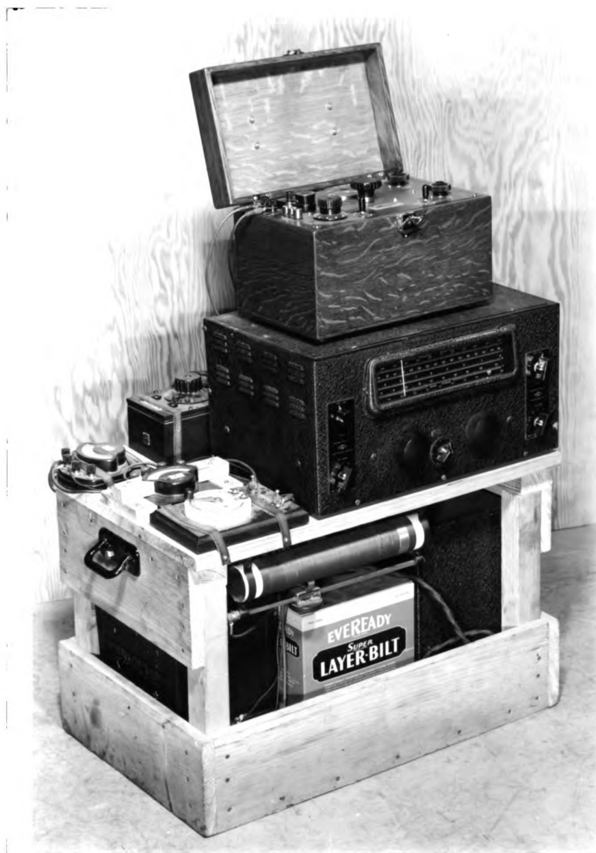
Fig. 3. Field Intensity Meter.
