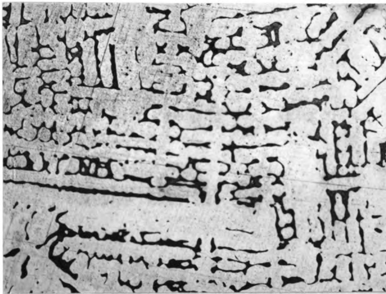
Solution heat treated at 1450°F for 4 minutes 100X
