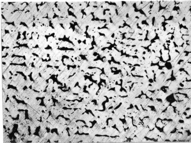
Solution heat treated at 1450°F for 16 minutes 100X
