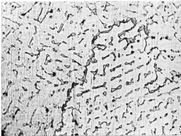
Solution heat treated at 1450°F for 16 minutes and aged at 800°F for 4 minutes 100X
