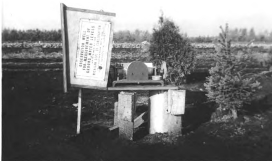
Figure 8 - Stevens type-F recorder in operation over long well, recorder shelter tilted back
