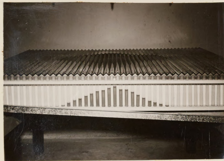
Fig. 19. Photo Single Nozzle Uniform Pattern.
