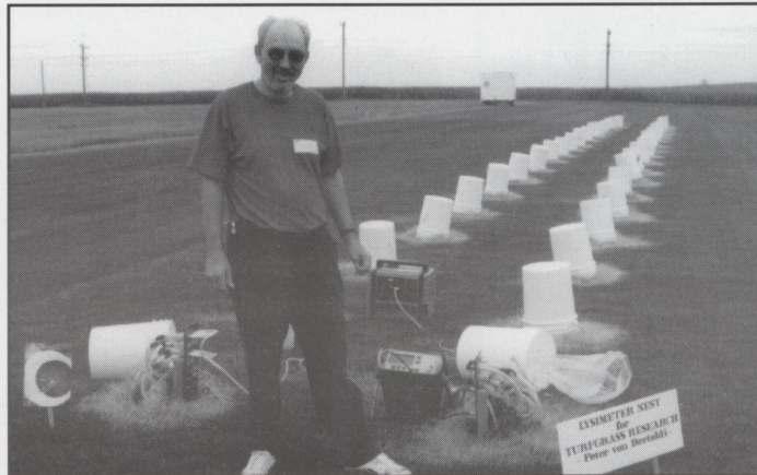
Peter Von Bertoldi - New lysimeter for studies of water and chemical management on turf
