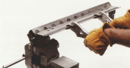
2 holes are machine punched in each bedknife and aligned with 2 dowel pins affixed to the bedknife bar to allow precision installation
