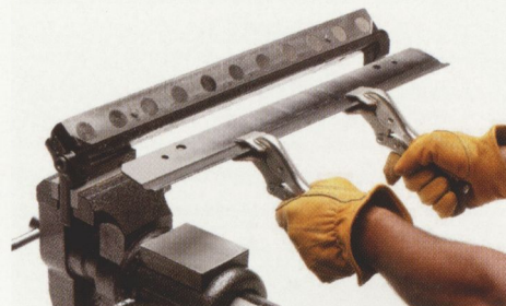
The high quality bedknife is installed with 2 special Mag-Knife vice-grip pliers
