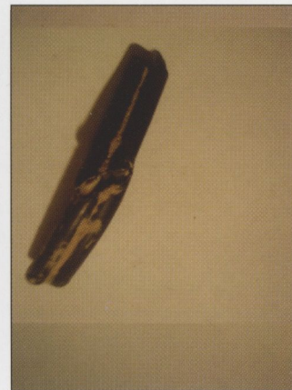
Nick in wire causing non-operation
