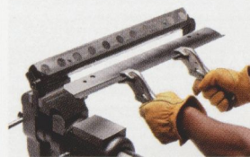
The high quality bedknife is installed with 2 special Mag-Knife vice-grip pliers
