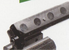
The New Mag-Knife bedbar after installation of rare earth magnets which hold the bedknife in precise position with uniform pressure.
