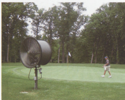
Figure 1. An example of a fan installed to increase air movement.
