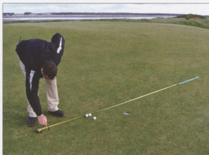
Measuring ball roll distance with a Stimpmeter days before the St. Andrews Links Trophy.
