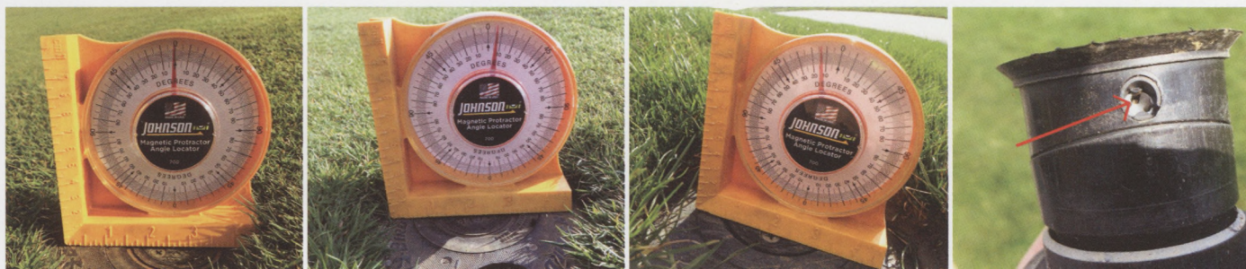
Top: Can catch test. (Credit: Jeff Stauffer); Bottom (l-r): Portable angle finder shows varying degrees of sprinkler heads from perfectly level to severely off level. Nozzle with particulate blocking upper outlet. Opposite: Sprinkler too low (depth greater than riser height). (Credit: Cam Shaw)
