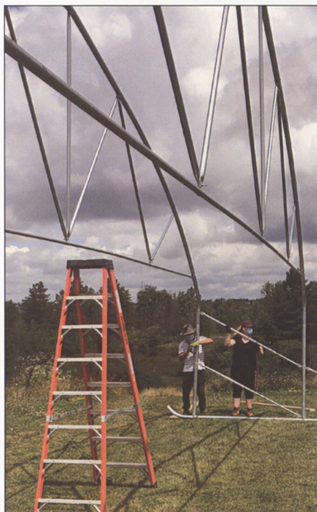
Grad students Corey Flude and Jaber Husiny seen here raising the scaffolding-like rain-out device over the TWCA Kentucky bluegrass trial plots.
