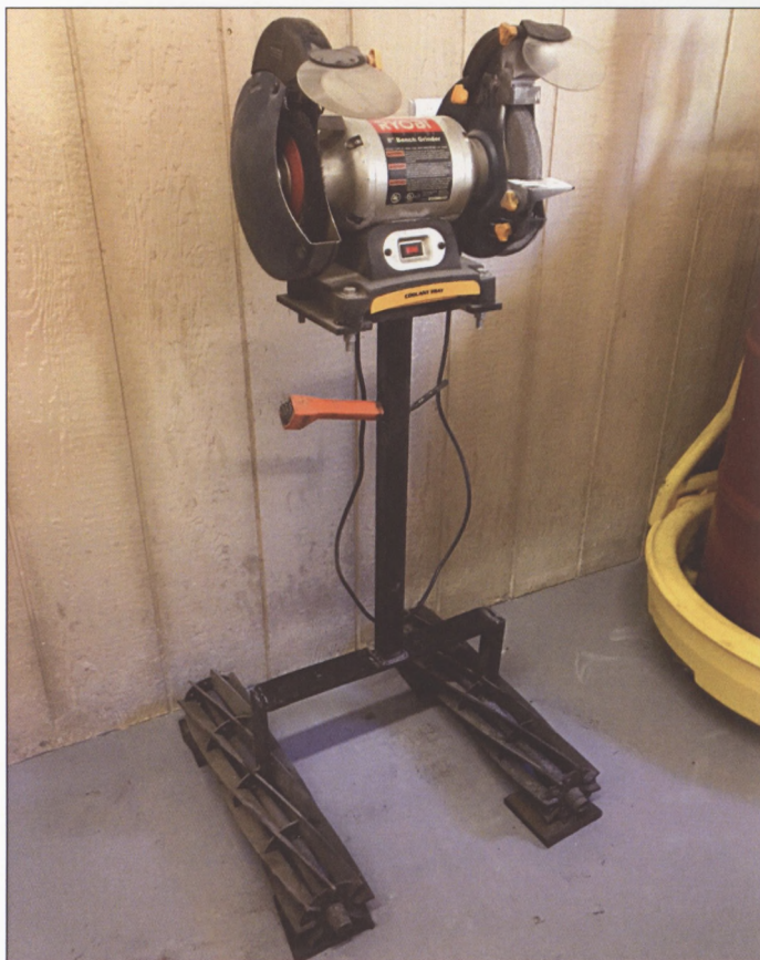
Resuing old reels to make a grinder stand.
