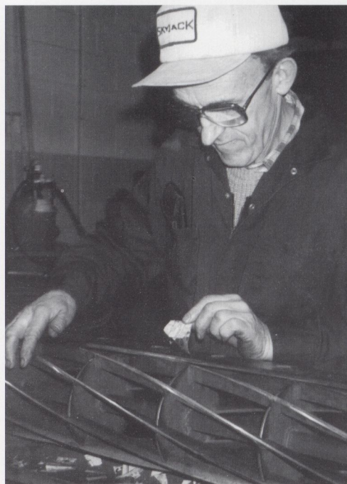
One of Gord's simple acid checks for sharpness, and minimal gapping, is sliding a few slips of the daily newspaper between the turning blades.
