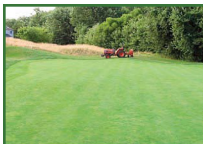
Tractor mounted or pull behind blowers can increase airflow around pocketed greens under stress.
