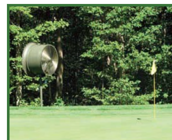
Oscillating fans may be necessary if trees/brush cannot be removed around pocketed greens.
