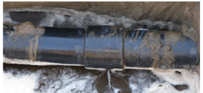
A typical join failure of a Fairway lateral pipe. The weld which is 40 years old has simply split. There can be up to 50 joins on each fairway vulnerable.
