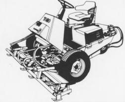
The Toro\* Turf Pro 84 is an all hydraulic triplex that gives you the right clip for the right height of cut and type of grass. All three reels and wheels are hydraulically powered, reducing maintenance time
