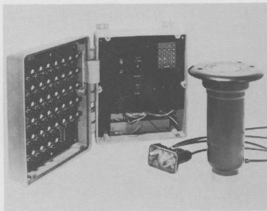
THE PRINCIPAL COMPONENTS for Toro's new low cost method for converting a golf course manual system to automatic irrigation are, left to right, the central controller, the cyler and, to replace the quick coupler, a valve-in-head gear-driven rotary sprinkler. The sprinkler shown is a Toro 670, which covers a full circle up to 204 feet in diameter.
