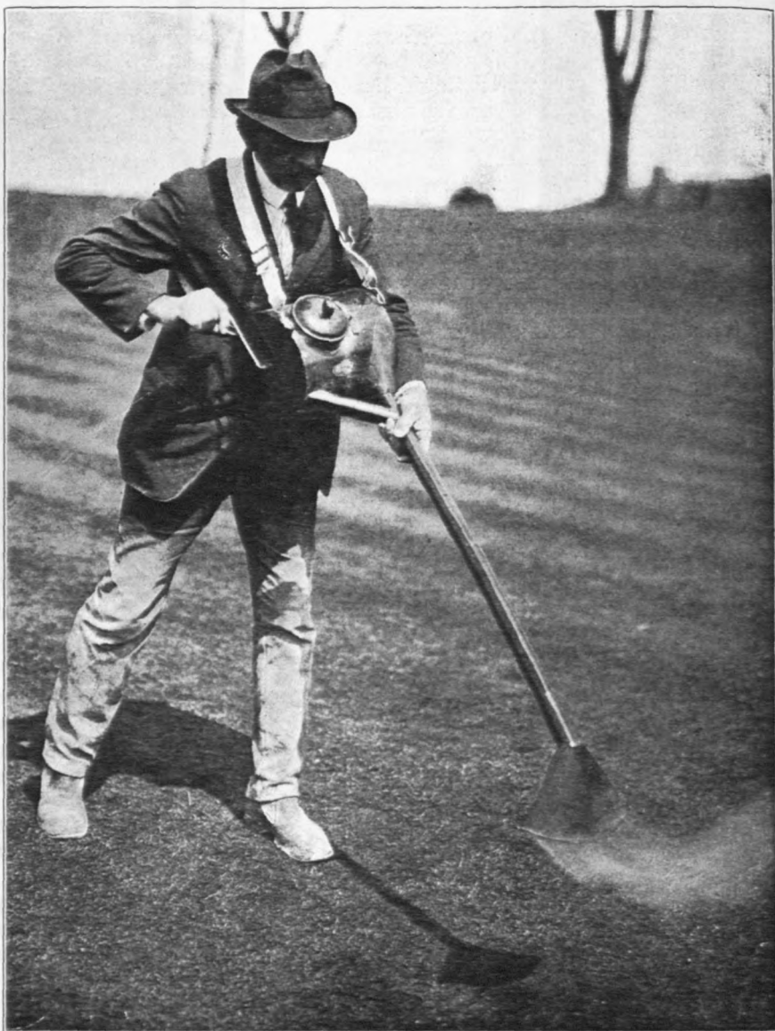
Fig. 1. A dust-gun used for applying Bordeaux powder to a putting-green.
