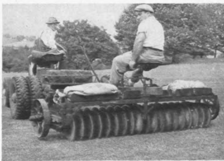
2. Rear view, carrying wheels off the turf. Machine cuts six-foot swath.
