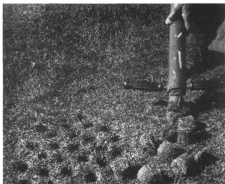
Plugs being emptied from tool. The magazine holds 24 plugs. Plugs of unsatisfactory turf are removed with the same tool so that plugs of improved turf fit exactly. This is becoming a favorite method on tees, athletic fields, and lawns.
