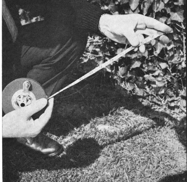
The steel tape, though an arduous task, is still one of the "recommended" methods for accurately measuring the course.
