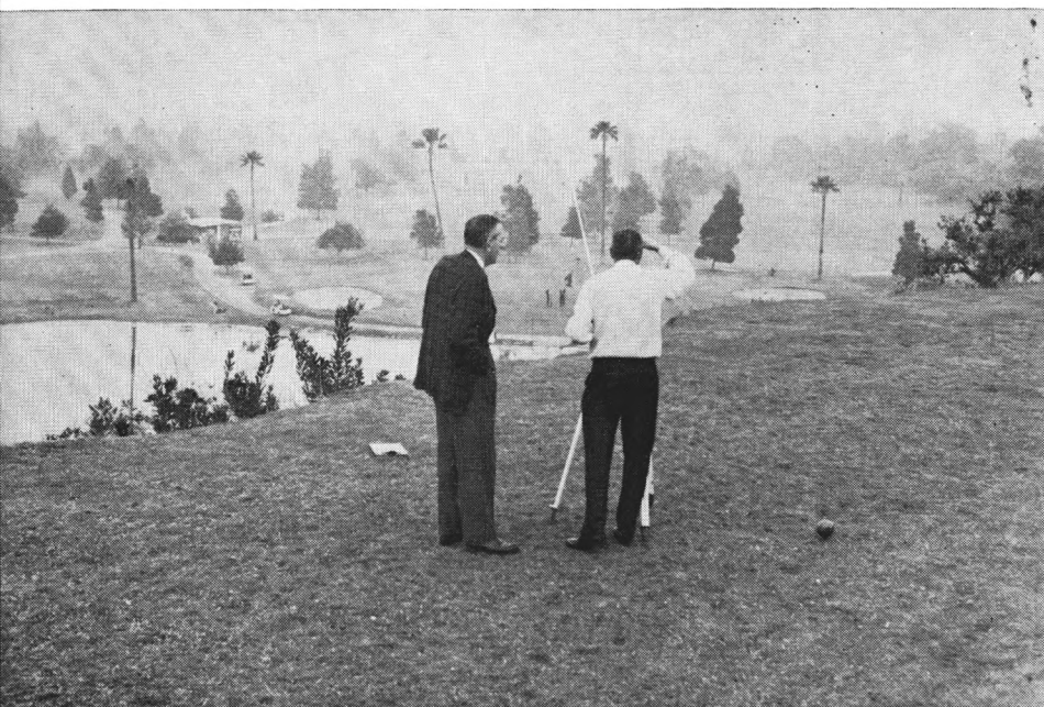
There is only one way to measure a golf hole of this kind accurately. The steep bank and lake below make the use of surveyor's instruments mandatory.
