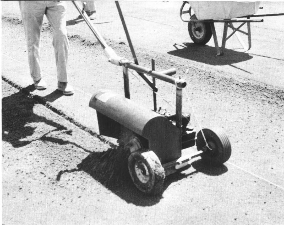
Putting green slots being cut with a modified commercial trencher. This was more effective than the chain saw method.
