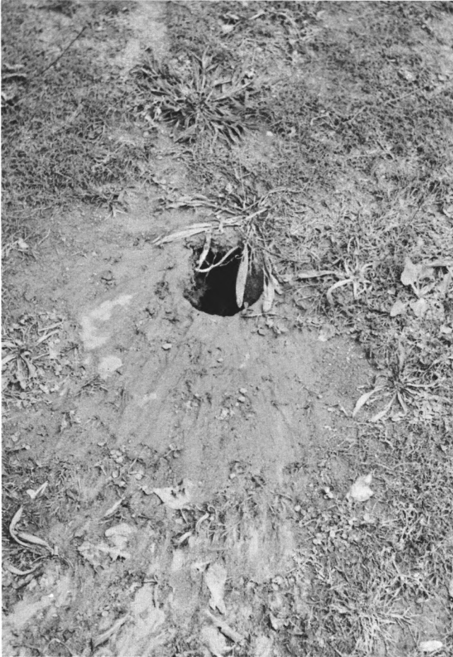
from installing a drain from the center of the bunker (left) where the first rain caused a blowout.
