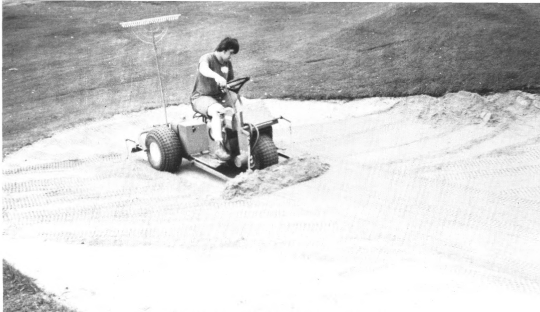
Turning a power rake into a small dozer.
