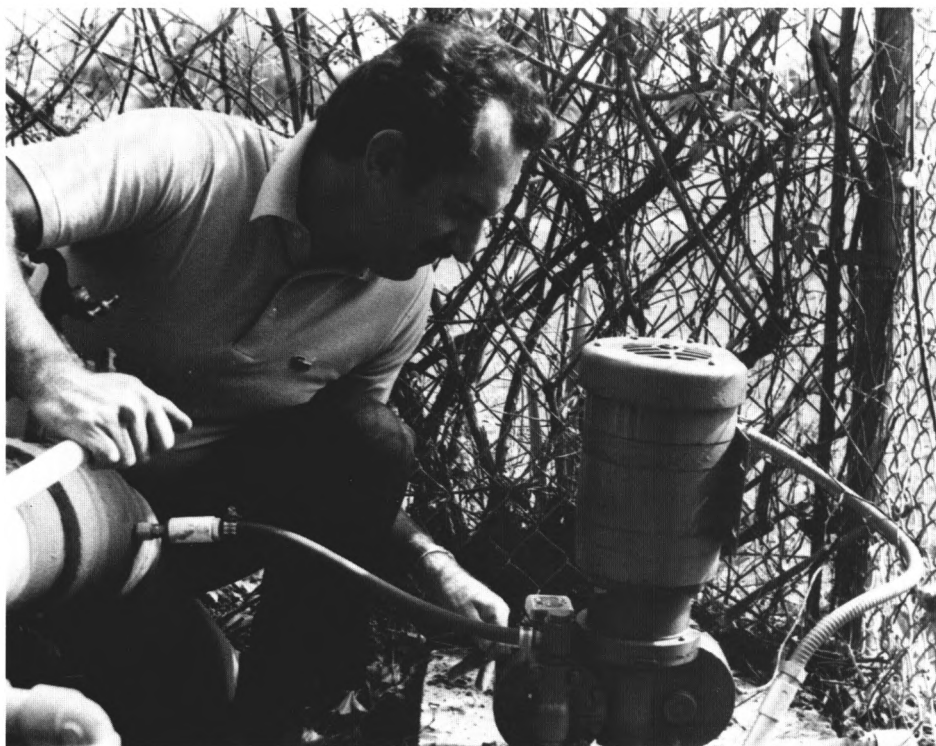
Superintendent Scott Sincerbeau adjusting the rate of fertilizer to be applied. This adjustment takes only a few seconds and is very accurate.
