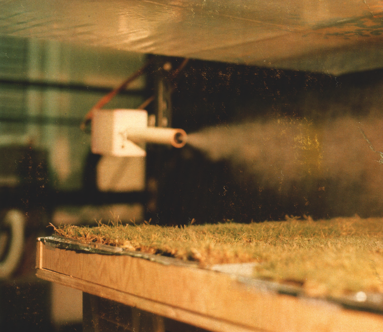
Figure 4. Electrostatic spraying of turfgrass under dielectric-barrier precipitator.
