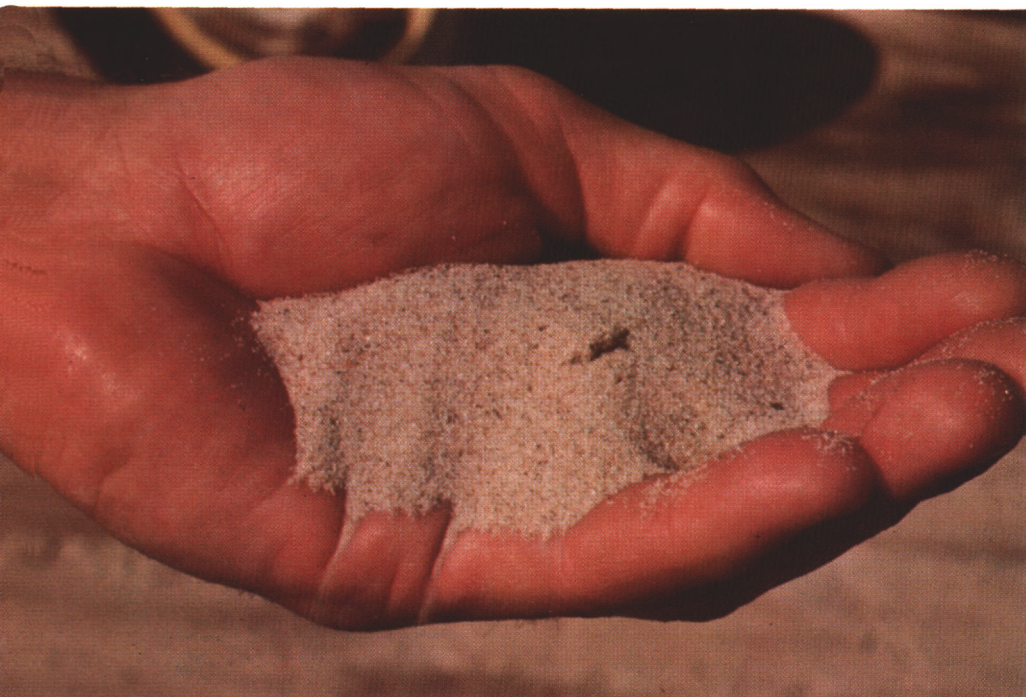
Preferred sand to use for topdressing greens — with particle size distribution ranging from 0.11 mm to 1.0 mm.
