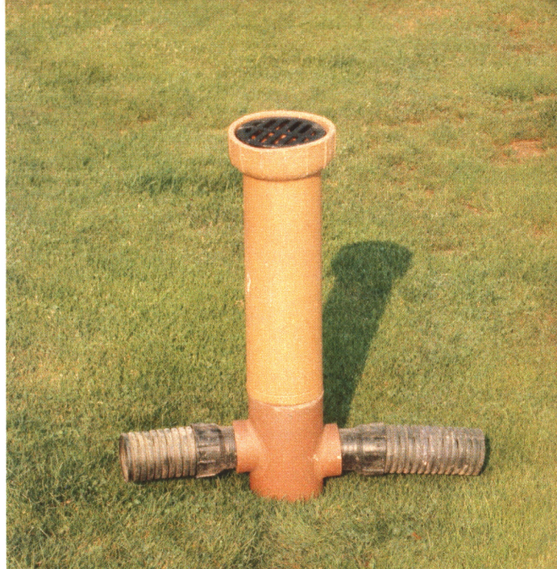
Surface risers with grates are installed in low areas for additional drainage and serve as visual checkpoints of water flow through drain lines.
