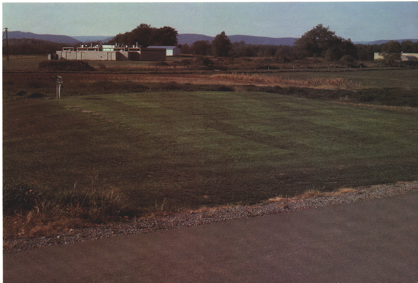
Figure 4. Construction of an outdoor system for testing turfgrass for allelopathy (plant toxins). The underground wooden framework was covered with plastic, filled with sand, and planted to Kentucky bluegrass, perennial ryegrass, and Poa annua, with the resulting grass cover.
