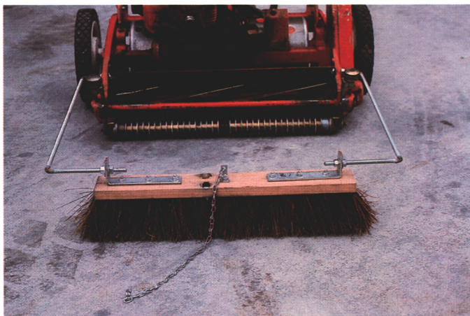
Brush made with threaded rod and floor broom.
