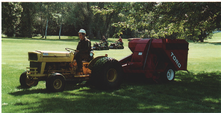
(Top) Clippings are broadcast into the roughs with manure spreaders which have an auger feed to a side or rear-discharge thrower.
