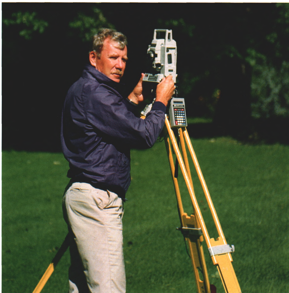
Setting up the laser and data collector.
