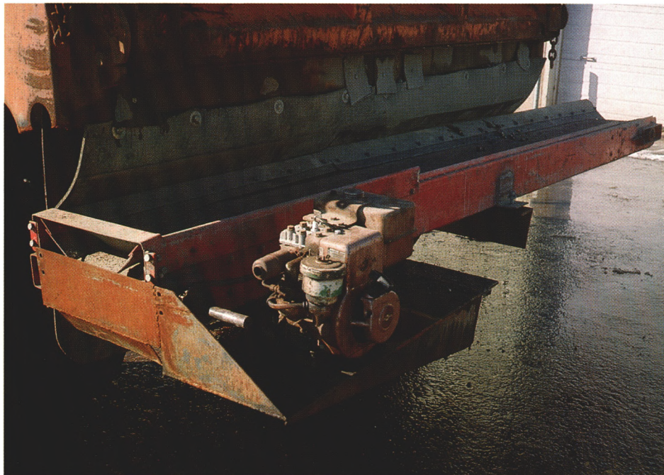
View of truck-mounted conveyor-belt device used to deliver crushed stone to drainage trenches.
