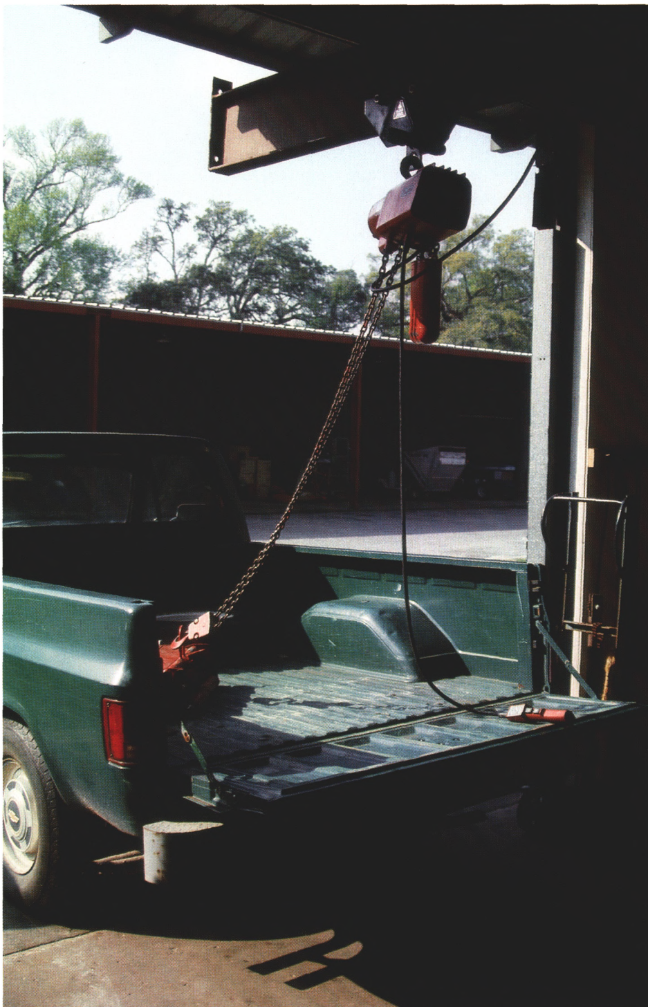
The movable electric hoist at Sea Island Golf Club can be conveniently used to remove mowers and reels directly from a pickup truck.
