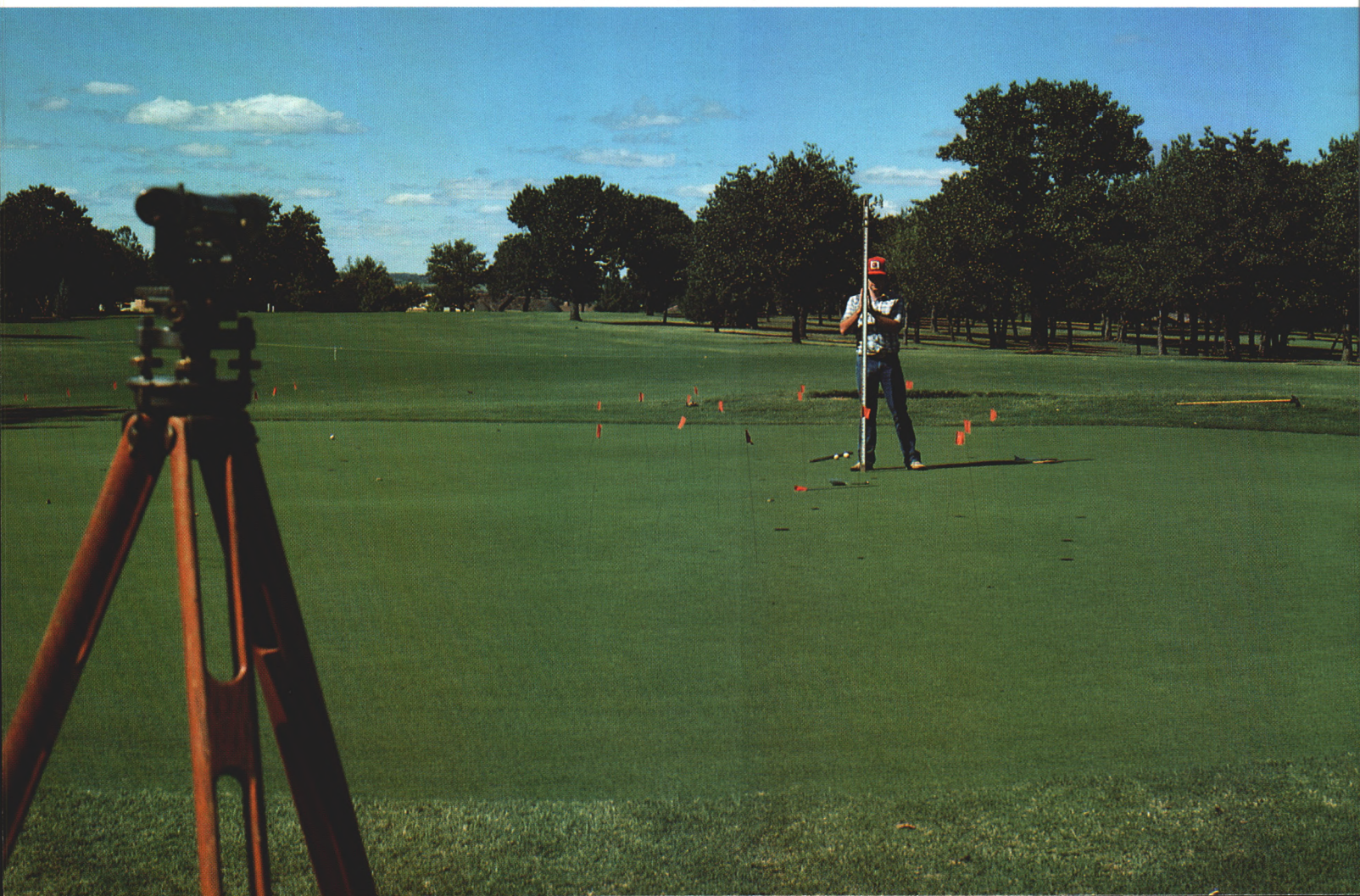
Figure 1. A formula (see text) was derived that corrects for slope in green speed readings. Here, the actual angles of inclination are checked before validation of the formula on the Stillwater (Oklahoma) Country Club.
