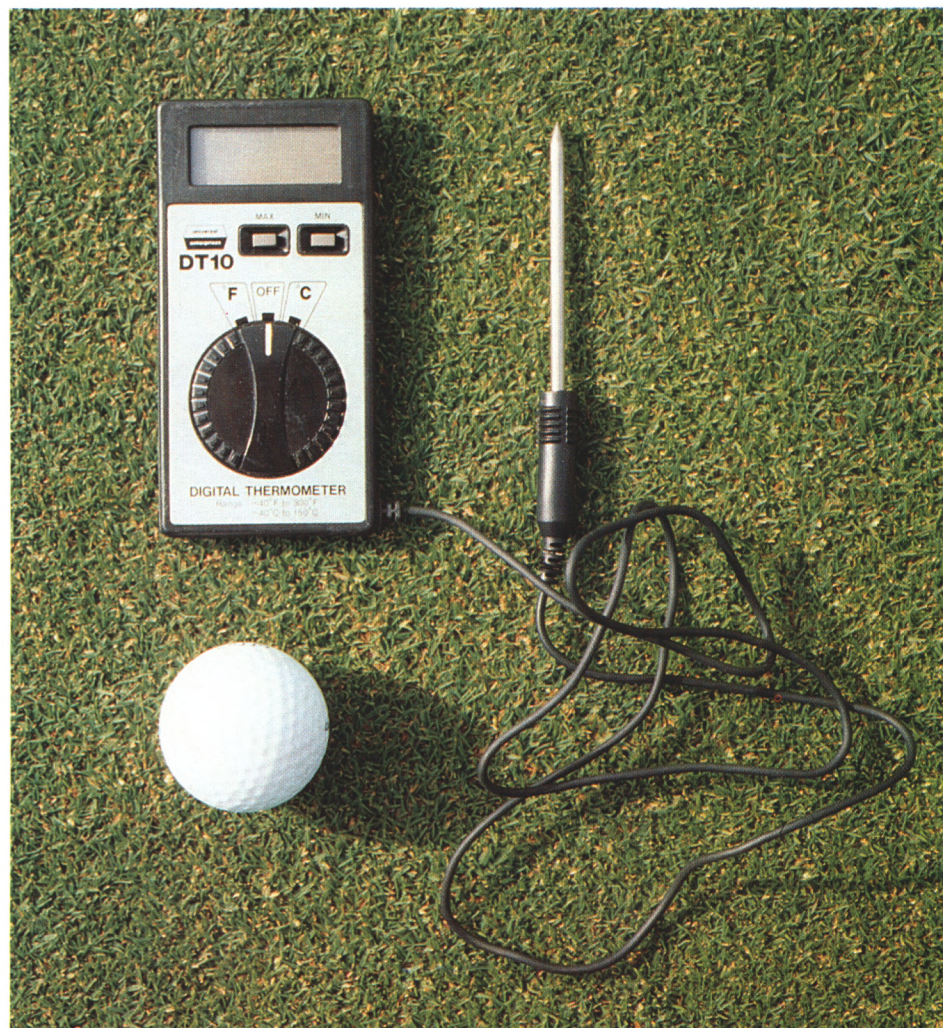
Digital thermometers, available through large electronic equipment suppliers, work well for monitoring surface temperatures because of their accuracy and mobile probe that can be placed directly on the surface.
