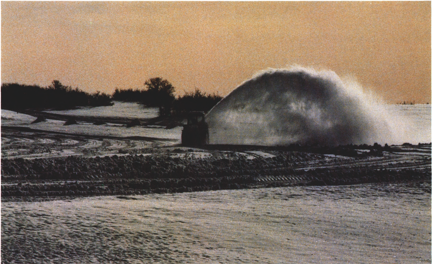
An early fall snowstorm in Colorado brought worry about the potential outbreak of snow mold. The quickest way to remove the snow was a snowblower set three inches above the turf.
