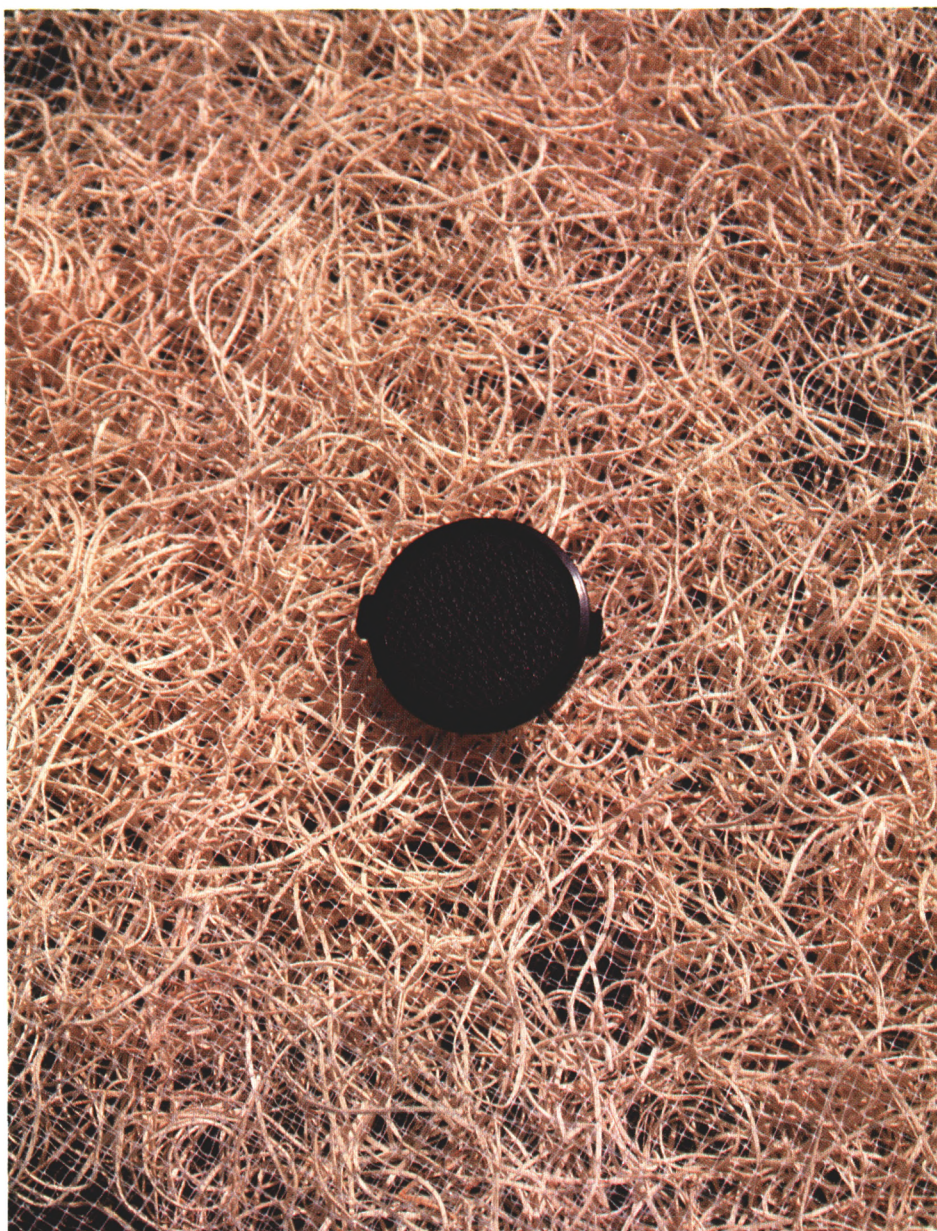
Aspen wood excelsior mats swell when wet, which provides more protection during freeze/thaw cycles than geotextile fabrics.
