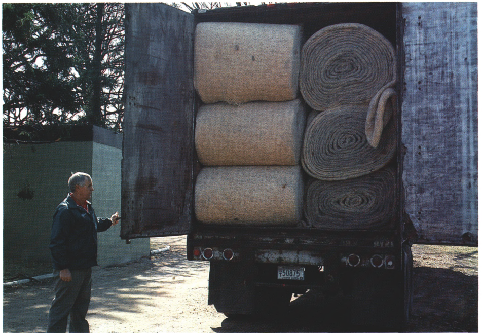
(Right) Excelsior mats are more difficult to handle than geotextile fabrics and require a considerable amount of storage space.
