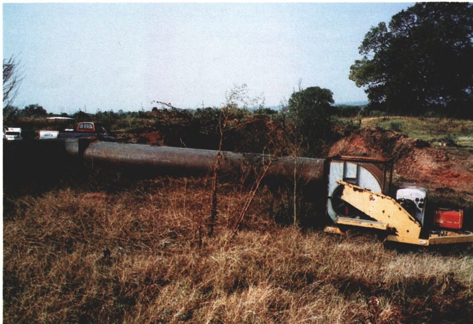
Constructing a forced-air incinerator for burning brush solved Southern Hills Country Club's problem of what to do with an overabundance of tree brush after an extensive tree improvement program was implemented.
