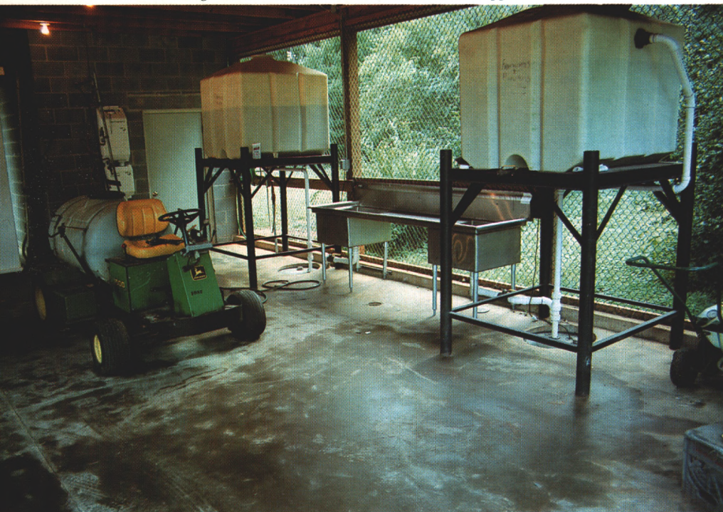
Elevated rinseate storage tanks hold rinseate to be used in the next application.
