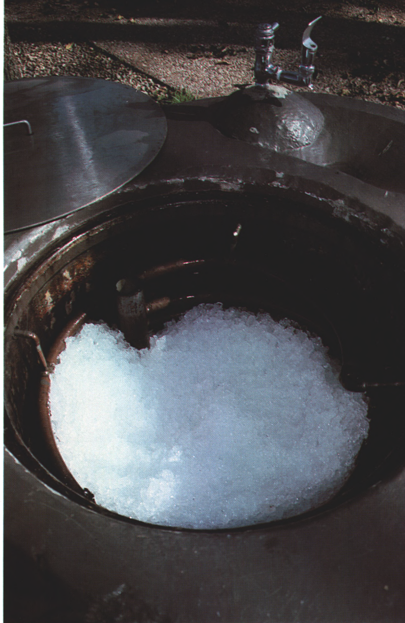
As the water travels through the copper coil, it is rapidly cooled by the ice.
