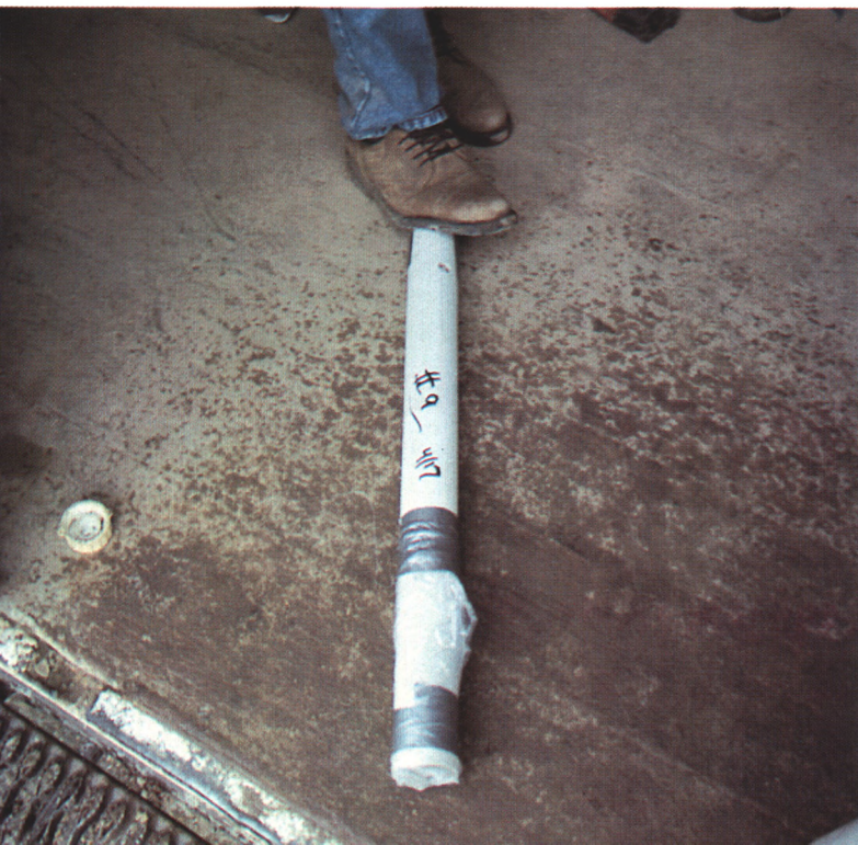
The best way to examine a soil's physical properties is by submitting an undisturbed soil core. To aid in sampling, a metal rod can be inserted through the end of the PVC sampling tube to help remove the pipe from the soil. Clearly identify each sample with as much information as possible. Securely tape the ends of each sample tube to prevent soil shifting.
