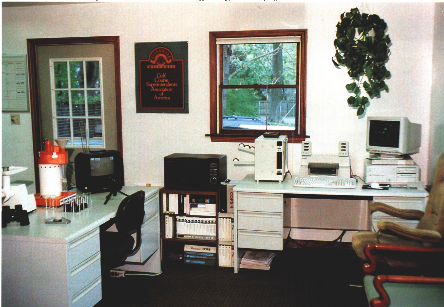
The Old Westbury Golf and Country Club uses in-house near-infrared spectral (NIRS) analysis to measure essential nutrients in leaf tissue. The results are used to modify the turf fertilization program.
