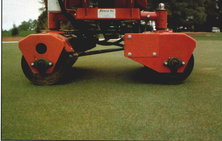
Compaction potential of various roller units can be compared by calculating the roll factor, which includes the unit weight, length of the rollers, and the diameter of the rollers in the equation.
