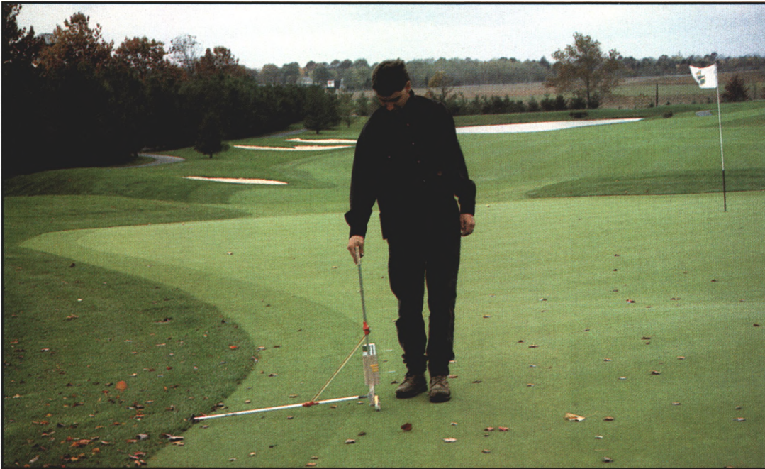
(Above) Originally two paint guns were used to mark the collar width of each green. The tool is held together with PVC pipe, but moves easily along flowing putting green contours.
