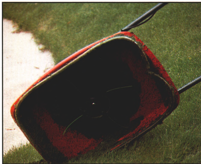
A Flymo is modified with \frac{5}{8} -inch vinyl tubing to elevate the machine for a greater height of cut.
