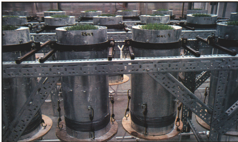
Research lysimeters generate data to form the basis of the KTURF model.
