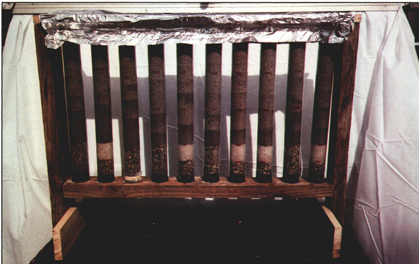
The research study investigated the moisture-holding capacity of a green constructed with and without the intermediate layer, using a rootzone mix with physical properties recommended by the USGA.
