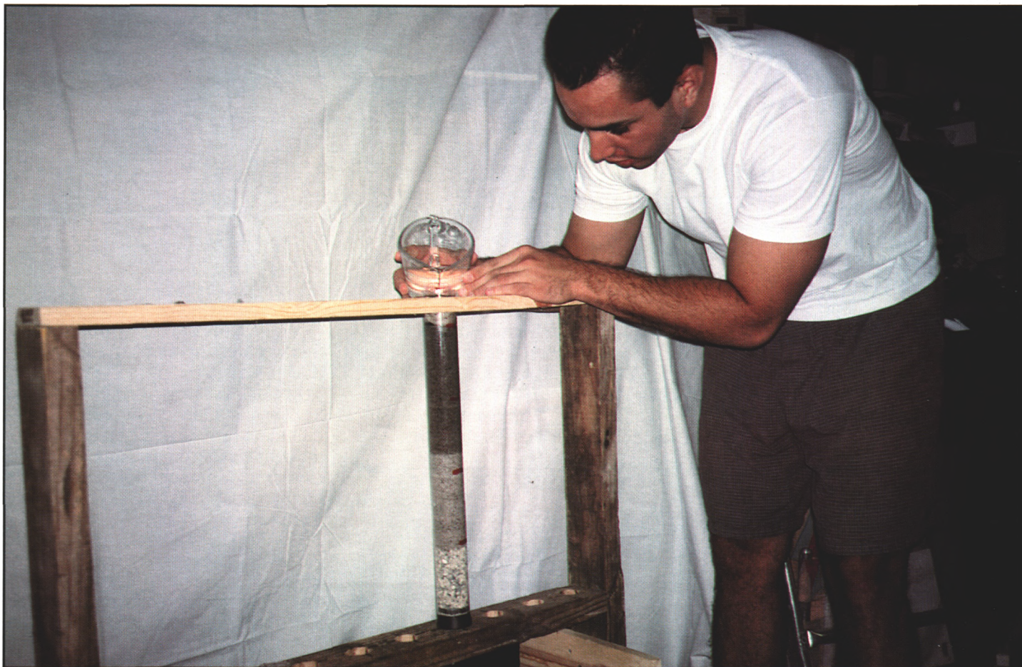
At the start of the study, each soil column was saturated with water before calculating the moisture content.
