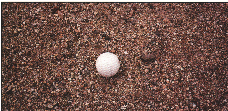
Evaluating the particle size range of the sand for bunker use is an important component in the selection process. A coarse sand will impact maintenance and playability.
