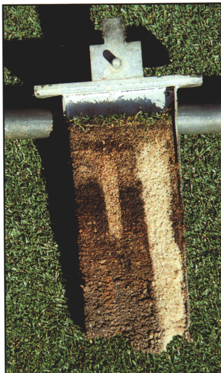
Layers in the green profile severely restrict internal drainage and can even block it altogether. Conventional aerification may not be deep enough to fully penetrate a buried layer. Deep-tine aerification is the next step in solving the problem.
