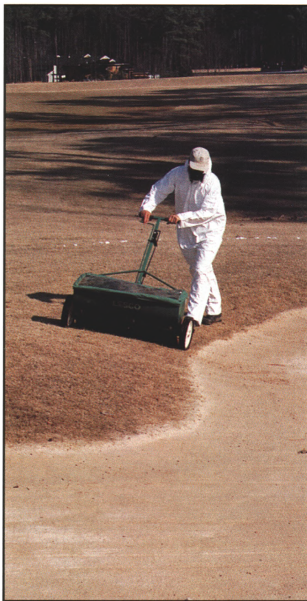
Drop spreaders and sprayers can be used in banding areas around impermeable surfaces and water resources to help reduce off-target movement of products.
